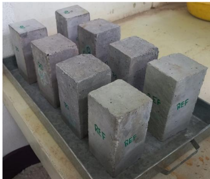
Figure 3. Specimens for the chloride penetration test.
